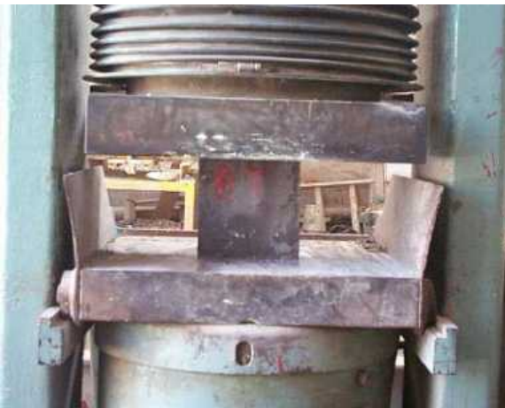
Figure VII.5 : essai de compression.
